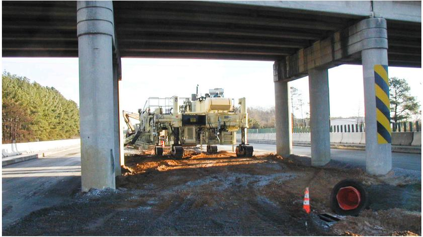
With the optional 90 degree steering and counter-rotation capability available on all G&Z four track slipform pavers, a G&Z paver with CDBI can walk and steer sideways through tight confines including bridge columns or other obstacle found on job sites.
