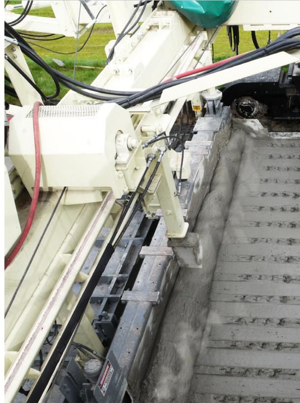
The Oscillating Correcting Beam (OCB) is a mechanical finishing device required behind the DBI to refine the concrete surface after dowel insertion. The precision built OCB includes bolt-on and replaceable wear plates on the bottom and leading edge as well as edge overbuild capability.
