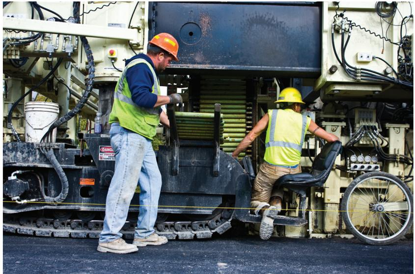
The CDBI is equipped with an operator station with seat designed for operator comfort and visibility. From the operator seat, the operator can easily reach the chain feeder and the CDBI control box.
